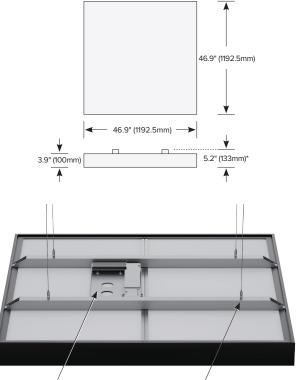
Power & Control tray (may be removed and mounted to ceiling) Suspended Mounting Option (LACC-SP-K)
