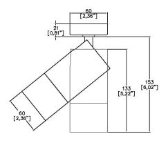
7100WD-LED-SMP Cut out Ø15mm
