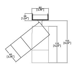
7100WD-LED-RMP Cut out Ø57mm
