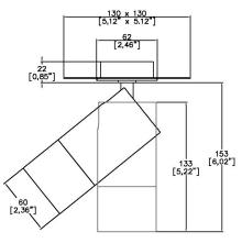
7100WD-LED-TMP Cut out Ø57mm
