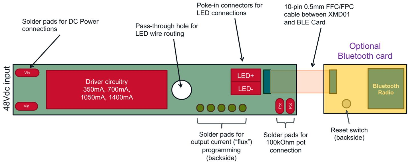
Figure 2: XMD wiring diagram
