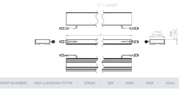
Provided data are typical values. Due to tolerances of the production process, figures for light output, electrical data etc can vary up to 10%. The Tc-point must be
