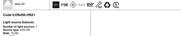
Watt: 15.4W Lm: 2235lm Lm/W: 145lm/W Kelvin/CRI: 4000K / >90 SDCM/L90 B10: < 3 / 50000
