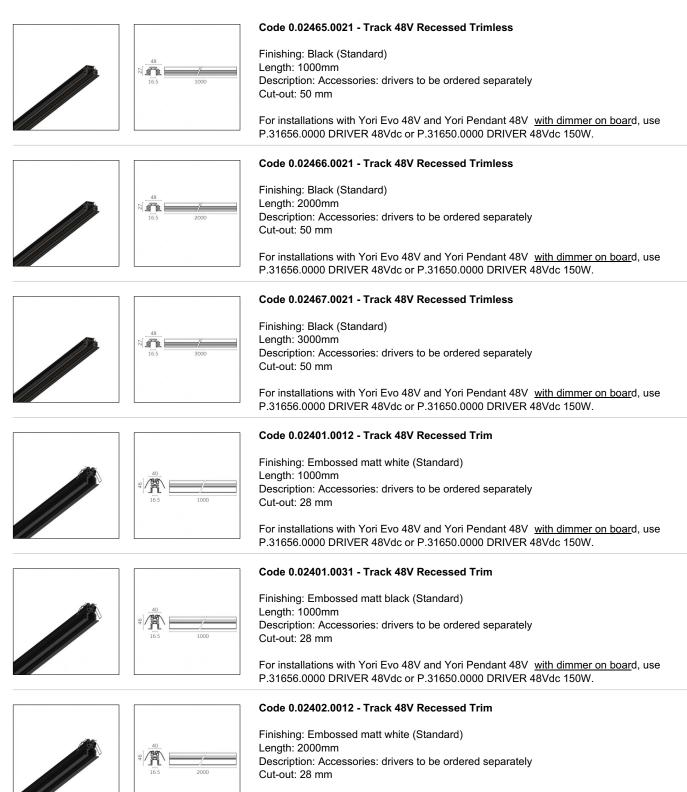
For installations with Yori Evo 48V and Yori Pendant 48V with dimmer on board, use P.31656.0000 DRIVER 48Vdc or P.31650.0000 DRIVER 48Vdc 150W.
