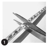
Handle strip with care. Cut with sharp scissors or snips on the dotted lines only.
