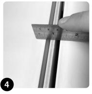
Fit the masked Groove Light into the channel taking care to set the product to the correct depth with relation to the channel.
