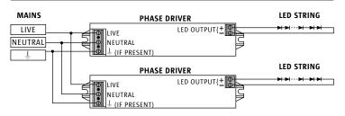
\* Diagram is indicative, check terminal locations on your driver before wiring
