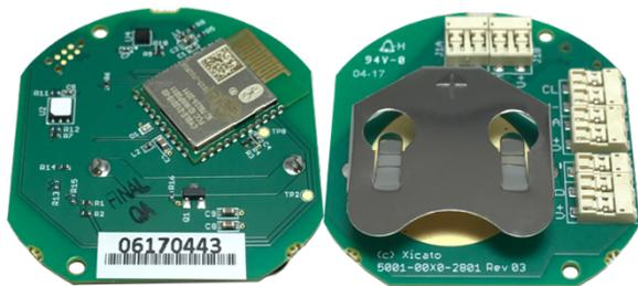
Figure 4: XIS02-B1THXYY Spider sensor body, top and bottom, showing connectors for external sensor elements
