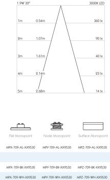
MPS-709-W/H-XX9530 For 3000K Substitute XX with 30 | For 2700K Substitute XX with 27
