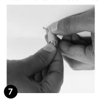
Tighten the Suspension Screw in a clockwise direction.
