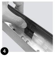
Attach black tape on inside of housing (both of up and down)
