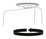
15 Ensure that the monopoint head studs locate securely in the mounting ring hooks, as shown below.
