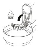
PAGE 6 PAGE 7 Unscrew lamp screws and remove the lamp connectors.
