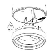
3 Unclip accessory holder and dispose of lamp correctly. To install a new lamp, reverse this process making certain lamp connectors are secured tightly to ensure a good connection and to avoid damage.
