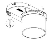
4 Insert the bezel ring over the snoot and clip into place over the accessory ring to lock the assembly together. Reattach the assembly to the DR8 spotlight.
