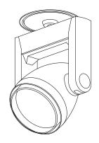
The monopoint fixture requires a minimum clearance distance of 200mm above and around the mounting point and a maximum ceiling material thickness of 50mm.
