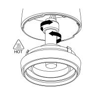
4 Unclip accessory holder and dispose of lamp correctly. To install a new lamp, reverse this process ensuring lamp is secured tightly.
