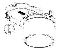
4 Insert the bezel ring over the snoot and clip into place over the accessory ring to lock the assembly together. Reattach the assembly to the DR8 spotlight.
