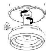
4 Unclip accessory holder and dispose of lamp correctly. To install a new lamp, reverse this process ensuring lamp is secured tightly.
