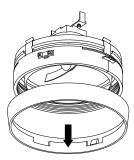
The accessory holder can hold up to two lenses, depending on the lamp type.
