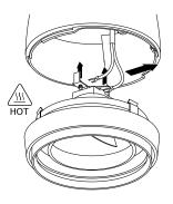
Unclip accessory holder and dispose of lamp correctly. To install a new lamp, reverse this process making certain lamp connectors are secured tightly to ensure a good connection and to avoid damage.
