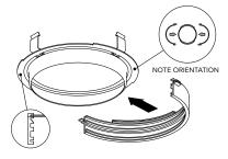
Insert the snoot into bottom slot of the accessory ring, as shown and bring the two halves of the ring together.
