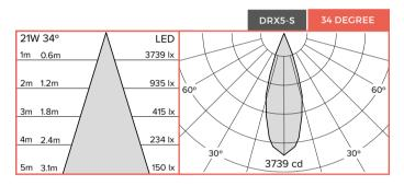
PEAK INTENSITY: 3739 CD BEAM DIAMETER AT 10M: 6.1M
