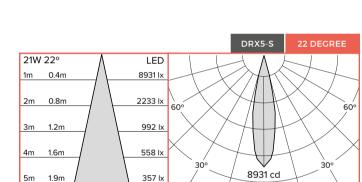
PEAK INTENSITY: 8931 CD BEAM DIAMETER AT 10M: 3.9M
