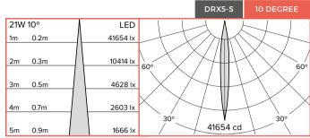
PEAK INTENSITY: 41654 CD BEAM DIAMETER AT 10M: 1.8M LX AT 10M: 417 LX
