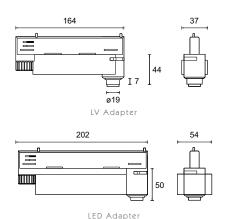
The Eutrac Adapter incorporates the Jack Plug connector to retrofit Precision Lighting's luminaires to existing mains voltage track systems. All of Precision Lighting's Jack Plug luminaires are compatible with the Eutrac 3-circuit track adapter. The adapters contain a dimmable 20-50VA transformer for use with Low Voltage luminaires. The LED adapter contains a 24V 20W PSU which is non-dimmable as standard.
