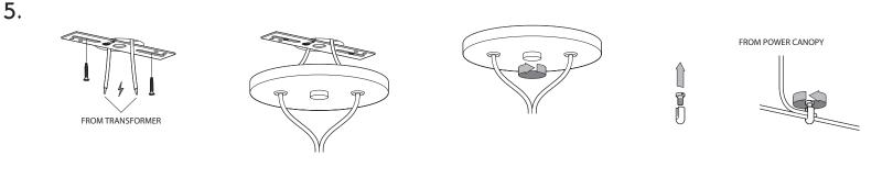
**NOTE** when installing ceiling brackets, be sure to align the pillar with the system before drilling holes to ensure the bracket will line up correctly when installed.
