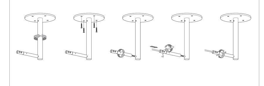
**NOTE** when installing Horizontal Standoff, be sure to align the pillar with the system before drilling holes to ensure the bracket will line up correctly when installed.
