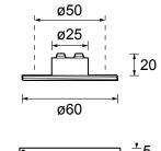
The Flat Monopoint uses Precision Lighting's Jack Plug system recessed into a discreet ceiling plate, with power being fed from a remote or local transformer. It is available in standard brushed aluminium, rubbed bronze, black and white finishes, with custom finishes available on request. Ideal for use with a BESA box.
