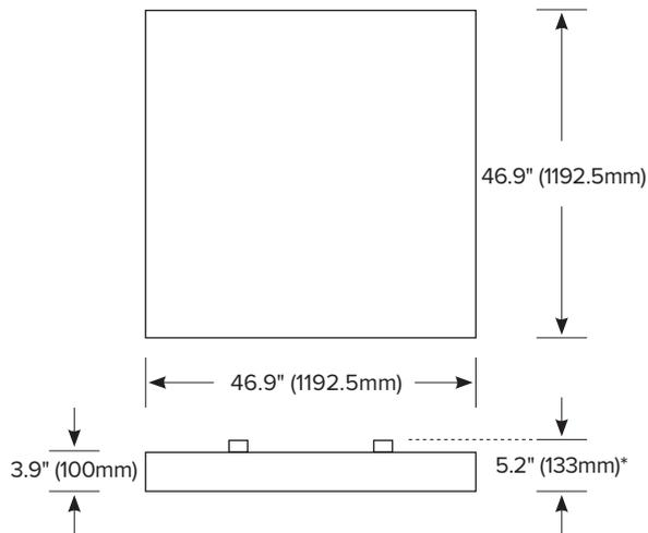
\*Surface Mount will have an opening of 1.3" (33mm) between the frame and the ceiling
