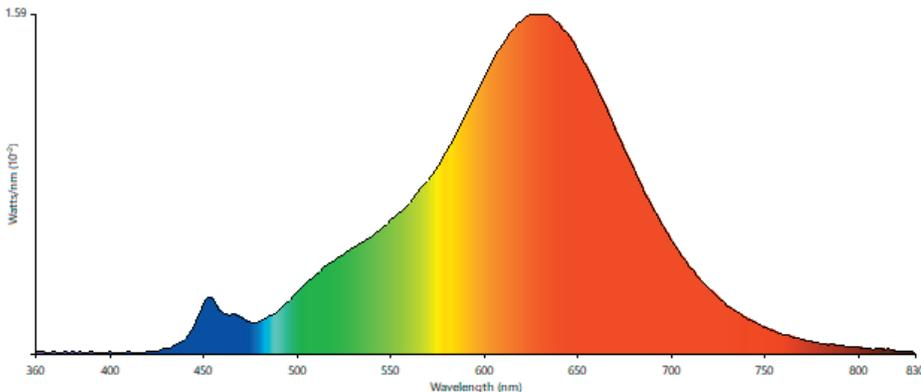
Testing was performed in accordance with LM-79-08.
