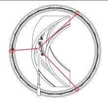
Screw the profile direct to the ceiling through the holes of the fixture
