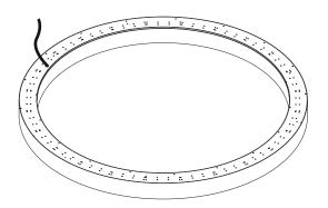
Pass the cable from the hole of upper part
