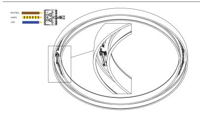
Connect the terminal block according the electrical instructions.
