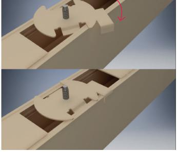
Push the protrusion of the 'gyra tool' while pressing the profile on the ceiling direction to lock it.
