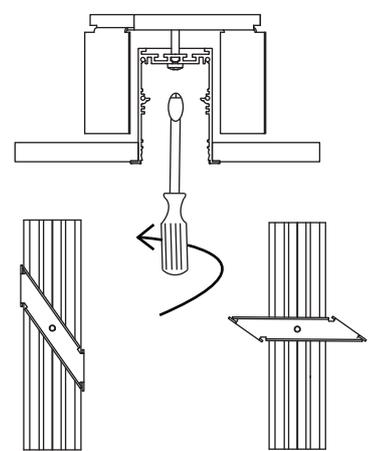
step 3\_ screw the fixation parts in order to 'open' the tool
