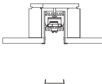
step 5\_ insert the heatsink with LED part and connect the fast terminal block
