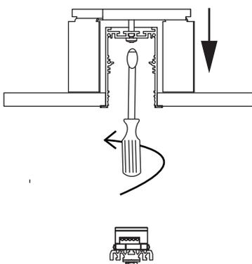
step 4\_ keep screwing to 'lock' the fixation part with the ceiling
