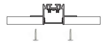
Screw from downside with self tapping screws.
