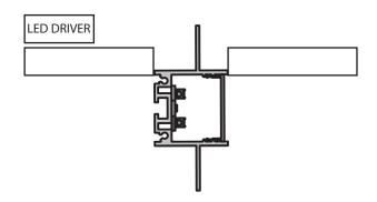
Connect the power supply to the terminal block The Driver must be installed remoted with potencially access after installation is shettled. Pass the fixture throu the hole
