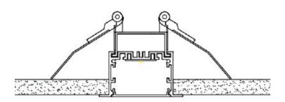
Press the springs and pass the profile through the false ceiling
