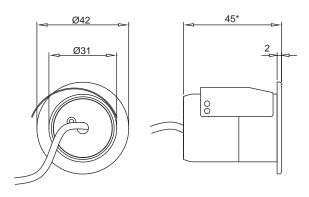
\* OR EITHER 58.5MM OR 73.5MM FOR DEEP SET VERSIONS DEPENDING ON HOW MUCH GLARE PROTECTION IS REQUIRED.
