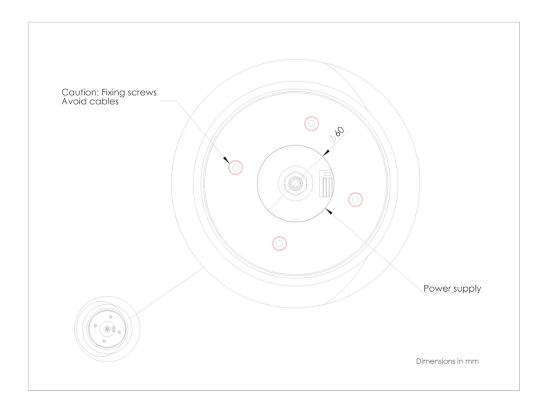
MECANICAL FASTENING: Make sure that the ceiling is straight. The fixing of the plate is realized with screws, see map. Use the appropriate method according to the materials on which it will bind. Lamp Weight: 7kg. Drill avoiding electrical cables.
