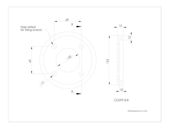
$\mbox{MOUNTING}$  : Mount the glass diffusing shade to the main structure following the attached plan.
