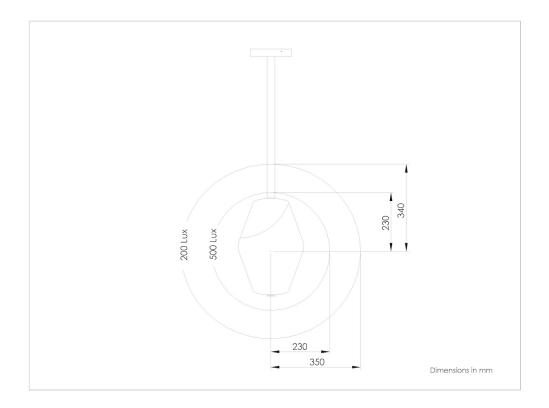
ELECTRICAL CONNECTION: Before connecting the fixture to the grid make sure it is not powered. Use the connector provided on the lighting. The lighting consumes 13W, is supplied without 350mA power supply and is designed to receive a remote power supply 350mA. We recommend the use of power supplies ELDOLED SOLOdrive 361/A witch allows optimal 0-10V and 0 to 100% dimming. It must be placed in an accessible and ventilated place.
