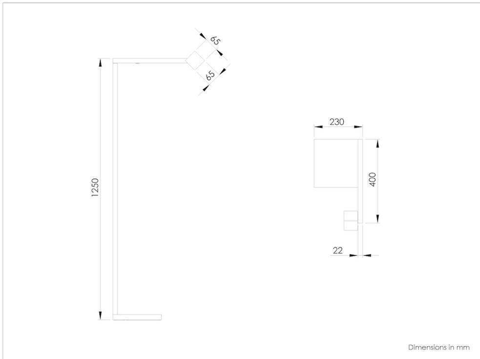
**FUNCTION :** The articulated design of the lamp makes it possible to place the light in the desired position on the caouch. Light is projected forward at an angle of 50°. Sources are equipped with honeycomb to prevent dazzling. The light output is 470Lumens equivalent to a 50W halogen spotlight . Light is produced by OSRAM brand LEDs 2700°K, with a CRI>80 and a yield of 90lm / W. Energy performance: A + .
