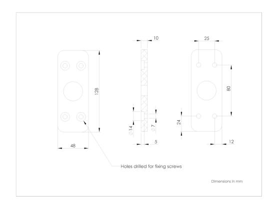
MOUNTING : After disconnecting the power supply, make the electrical connection using the supplied connectors and according to the polarity (red: plus, black: minus).Mount the diffusing shade to the plate using the screws provided following the attached plan.
