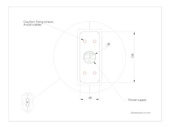
MECANICAL FASTENING : The fixing of the plate is realized with screws, see map. Use the appropriate method according to the materials on which it will bind. Lamp Weight: 4kg. Drill avoiding electrical cables.
