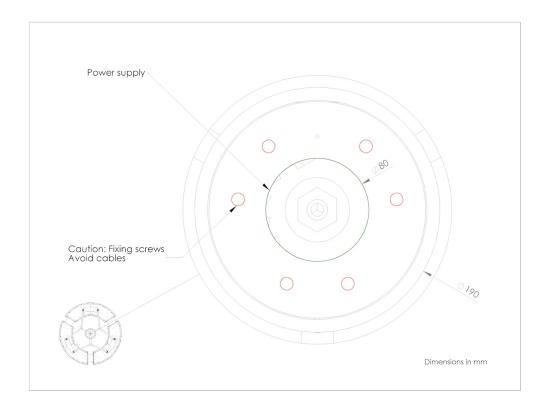
MECANICAL FASTENING : If necessary please reinforce the ceiling at the plate. Make sure that the ceiling is straight. The fixing of the plate is realized with screws, see map. Use the appropriate method according to the materials on which it will bind. Lamp Weight: 60kg. Drill avoiding electrical cables.
