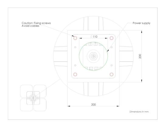
MECANICAL FASTENING: Make sure that the ceiling is straight. The fixing of the plate is realized with screws, see map. Use the appropriate method according to the materials on which it will bind. Lamp Weight: 50kg. Drill avoiding electrical cables.
